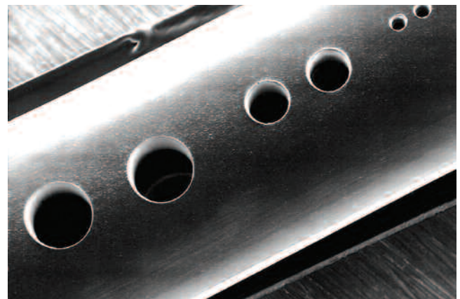
Figure 6. Both the diameter and shape of drilled holes can be controlled with laser system software.
