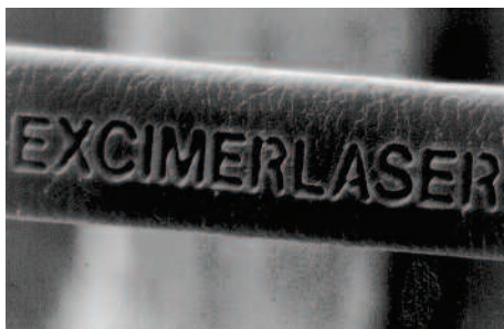
Figure 1. Excimer lasers can micromachine on objects as small and delicate as a human hair.
